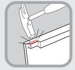
Extra instructions for Thin-Line Tile Vent: When used with a Quinn Lakeland Slate or Russell Galloway tile profiles, you may have to remove the side lock nib from the tile, as shown.
