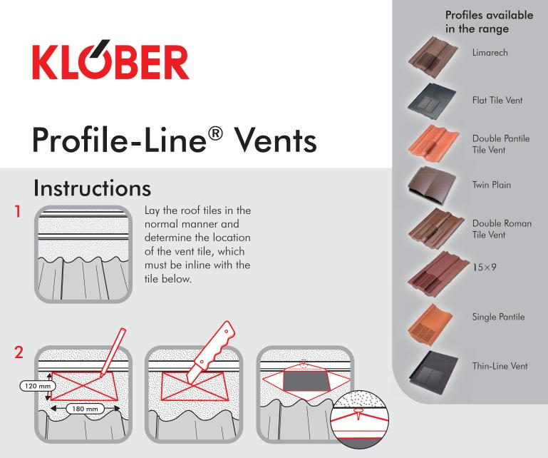
Mark a 120 mm x 180 mm wide rectangle on the underlay directly below the tile batten where the vent is to be fixed. Carry out a star cut within the rectangle and fold the four tabs back and secure the top tab to the tiling batten.
